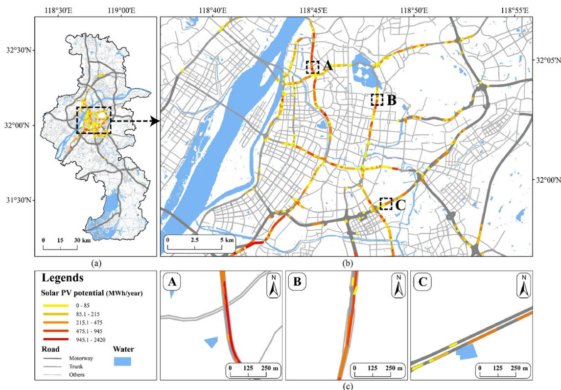
**Fig. 13.** Spatial distribution of the solar PV potential of planned noise barriers in Nanjing. (a) An overview of the solar PV potential of planned noise barriers in Nanjing with dash line box marked the part of the magnified area; (b) The magnified area in the main urban area of Nanjing; (c) The partial detail display of the marked three areas in Fig. 13 (b).
