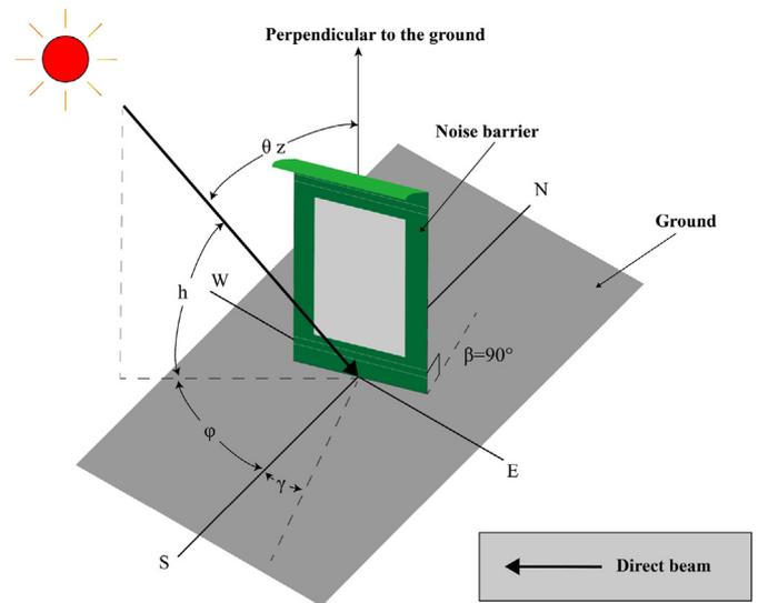
Fig. 8. Schematic diagram of the locative relationship between incident sunlight and a noise barrier, where  $\beta$  is the slope angle of the noise barrier,  $\gamma$  is the azimuth angle of the noise barrier,  $\phi$  is the azimuth angle of the sun,  $\theta_z$  is the zenith angle of the sun, and  $h$  is the altitude angle of the sun.
