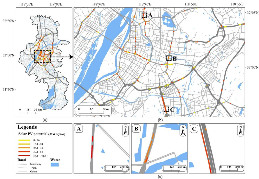
**Fig. 11.** Spatial distribution of solar PV potential of the existing noise barriers in Nanjing. (a) An overview of the solar PV potential of the existing noise barriers in Nanjing with dash line box marked the part of the magnified area; (b) The magnified area in the main urban area of Nanjing; (c) The partial detail display of the marked three areas in Fig. 11 (b).
