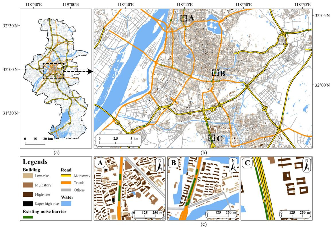
**Fig. 10.** The automatic detection result of existing noise barriers in Nanjing. (a) An overview of the spatial distribution of existing noise barriers in Nanjing with dash line box marked the part of the magnified area; (b) The magnified area in the main urban area of Nanjing; (c) The partial detail display of the marked three areas in Fig. 10 (b).
