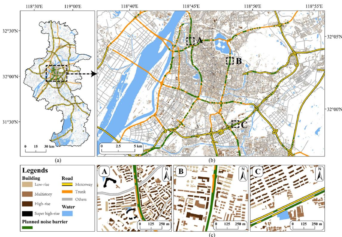
**Fig. 12.** Spatial distribution of planned noise barriers in Nanjing. (a) An overview of the spatial distribution of planned noise barriers with dash line box marked the part of the magnified area; (b) The magnified area in the main urban area of Nanjing; (c) The partial detail display of the marked three areas in Fig. 12 (b).
