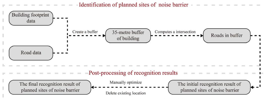
Fig. 6. Flowchart of the identification of the planned sites of the noise barrier.
